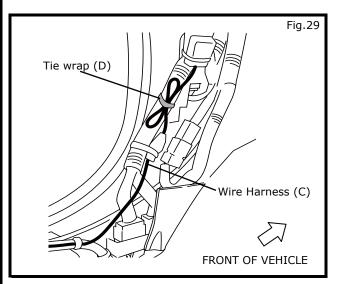
11) Attach excessive Wire harness (C) to the vehicle harness with Tie wrap (D) as shown in Fig.29.(1 place)
