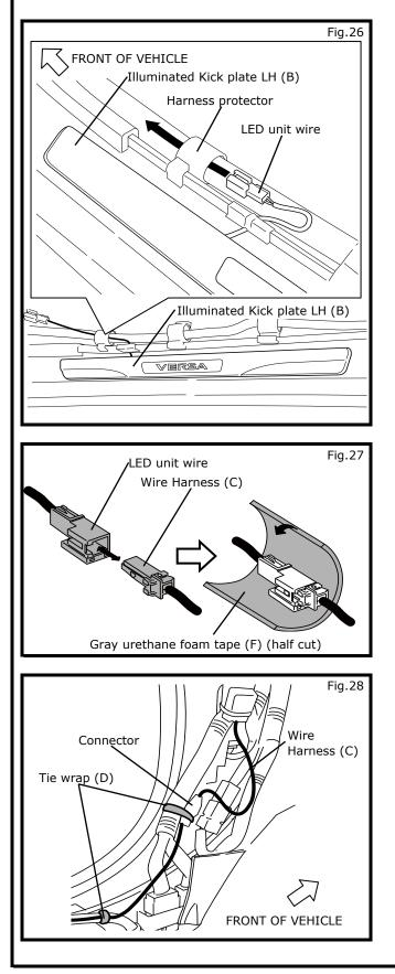
8) Route LED unit wire of Illuminated Kick plate LH (B) into harness protector as shown in Fig.26.
