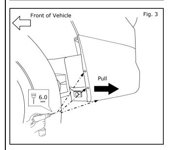
4) While pulling rear bumper outward, drill 6mm (1/4") holes at center of all scribe mark locations on bumper.
