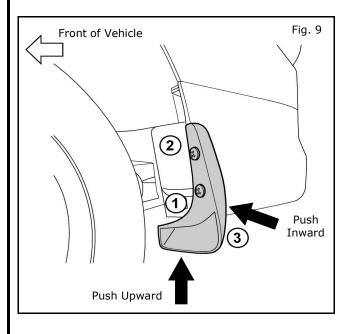
9) Push splash guard upward and inward towards vehicle and tighten three screws in sequence shown.
