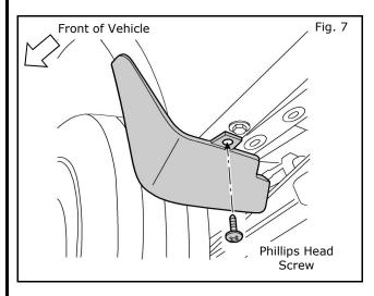
9) Align splash guard to vehicle and loosely install phillips head screw at bottom location.
