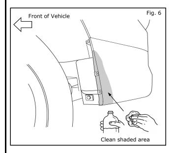
8) Clean installation surface (shaded area) with mild soap/water mixture.
