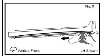
14) Beginning at rear of vehicle and moving forward, apply 15 lbs of pressure over entire part.
