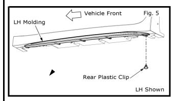
9) Mount LH molding to mud guard and install rearmost plastic clip.
