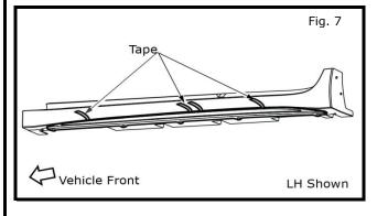
11) Remove and discard tape liner, pulling tape liner forward as shown. See Fig. 7.
