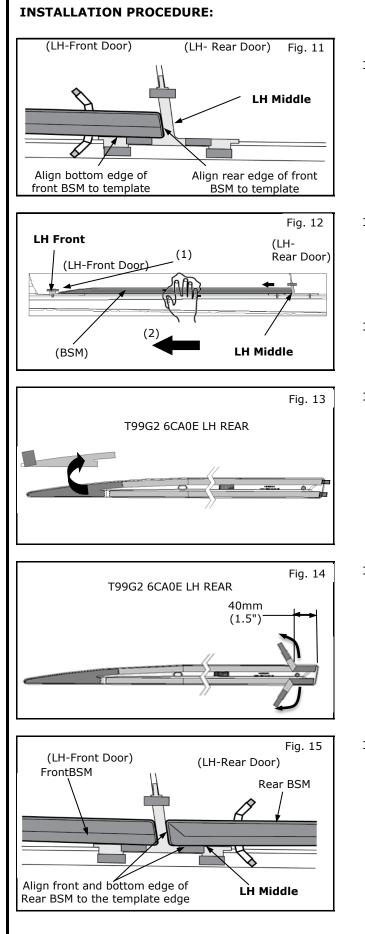
14) Align rear edge of Front Body Side Molding to the template edge as shown.
