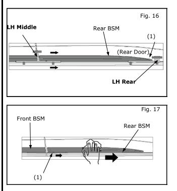
20) Align bottom edge of Rear Body Side Molding to top edge of rear template and press lightly into position. Slowly remove top & bottom tape liner from Body Side Molding.
