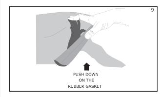
14. Push down on the rubber gasket with your thumb along the entire length to seat the rubber gasket correctly with the roof surface.
