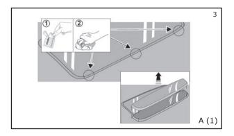
5. Remove the sunroof wind deflector, clean the roof at the 3 marked areas with alcohol wipe provided and wipe with a clean dry cloth.
