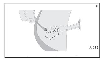
8. Identify the center metal clip, item E, as the longest of the three clips. Install this clip over the center abrasive resistant tape and hold it in place with masking tape. Install the remaining metal clips over the outer tape and hold in place with masking tape. Be careful not to bend the clips during installation. The clips should remain straight against the sunroof opening flange.
