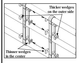
3) Using a T-20 Torx wrench, screw together the double wedges in the plastic upright cavity with the PT Screws as shown in the figure (double wedge thru-hole goes in the center and double wedge threaded goes on the outer side). Tighten to 2.3 N-m (20 in-lbf).
