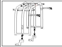
4) Lower the Bed Extender into the brackets by holding it in the vertical position. Also, have the Bed Extender in vertical position to remove from the brackets.
