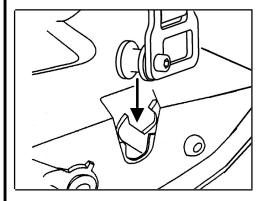
3) When the Bed Extender is at outward position, push down on the buckles to insert into tailgate latches. Tighten straps. To release, pull tailgate handle.
