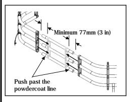
1) Slide the Extension Tubes evenly into the Left and Right Bent Tube Assembly.
