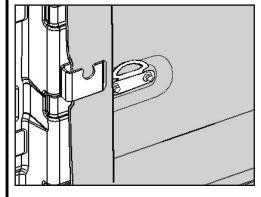
NOTE: The Bolt-On Brackets goes between the truck bed sheet metal and the bed liner.
