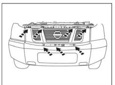
2) Install grille assembly from front of vehicle. Push clips into bolster and headlamps. Grille has 7 clips (4 top, 3 bottom) to the bolster and 4 clips (2right, 2 left) to the headlamps.
