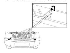
1) Open the hood and remove the production grille by turning 7 clips counter-clockwise ¼ turn and then pull grille forward.
