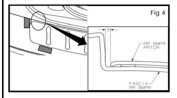
5) Confirm Bumper Protector location on vehicle with scale at first bead and mark location by applying tape on RR edge of bumper protector
