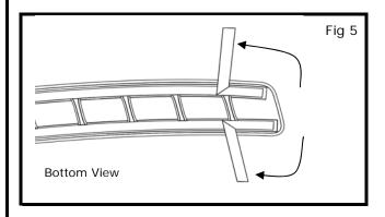
6) Remove part and peel approximately 30mm of all tape liners (RH & LH).
