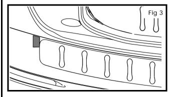
4) Apply tape at RH & LH edges of part.
