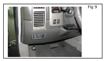
12) Move Drivers seat rearward most postion and apply parking brake to gain access to DASH LOWER as shown in Fig 9.
