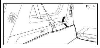
4) On both sides of liner, press weighted pouches into forward cup receptacles.
