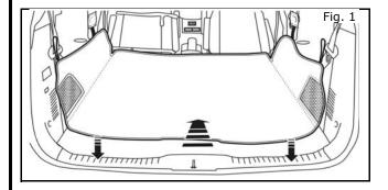
1) Open the rear door and fold down the third row seats. Slide cargo liner into vehicle and place front edge on top of the 3rd row seats.
