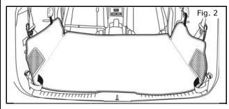
2) On both sides of liner, wrap elastic loops around lower cargo tie downs.
