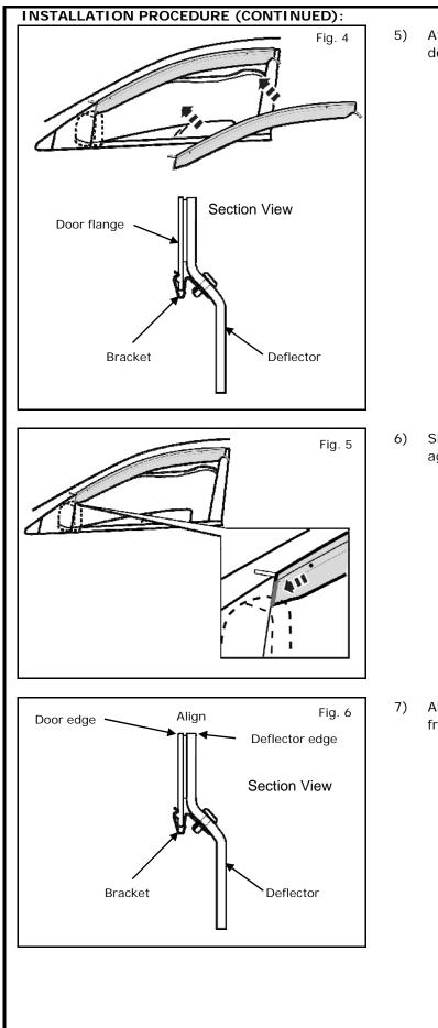
) Attach deflector to door by sliding brackets onto door flange.
