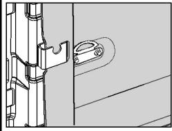
NOTE: The Bolt-On Brackets goes between the truck bed sheet metal and the bedliner.
