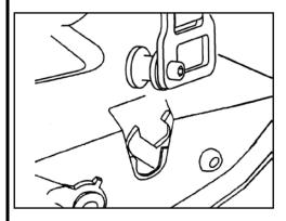
2) When the Bed Extender is at outward position, push down on the buckles to insert into tailgate latches. Tighten straps. To release, pull tailgate handle.
