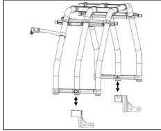
4) Lower the Bed Extender into the brackets by holding it in the vertical position. Also, have the Bed Extender in vertical position to remove from the brackets.
