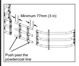
1) Slide the Extension Tubes evenly into the Left and Right Bent Tube Assembly.
