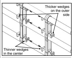
3) Using a T-20 Torx wrench, screw together the double wedges in the plastic upright cavity with the PT Screws as shown in the figure (double wedge thruhole goes in the center and double wedge threaded goes on the outer side). Tighten to 2.3 N-m (20 in-lbf).
