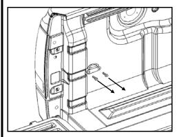
1) Remove the bolts that secure the tiedown hooks with a 12 mm wrench. **Do not** discard the bolts, retaining washers, and tiedown hooks.
