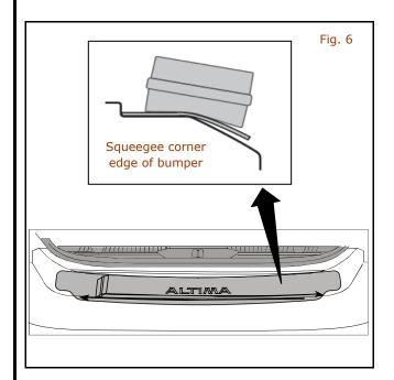
10) Firmly squeegee corner edge of bumper with three or four back and forth strokes in direction shown.
