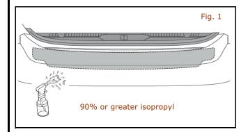
1) Using a clean lint free micro fiber cloth clean highlighted surface of rear bumper with 90% or greater isopropyl alcohol. Allow area to dry completely.
