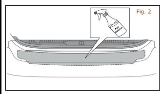
2) Spray highlighted bumper surface with application solution.
