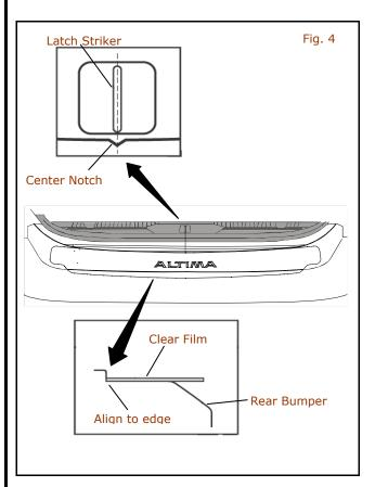
5) Align applique into position with notch to latch striker and film edge against bumper edge.
