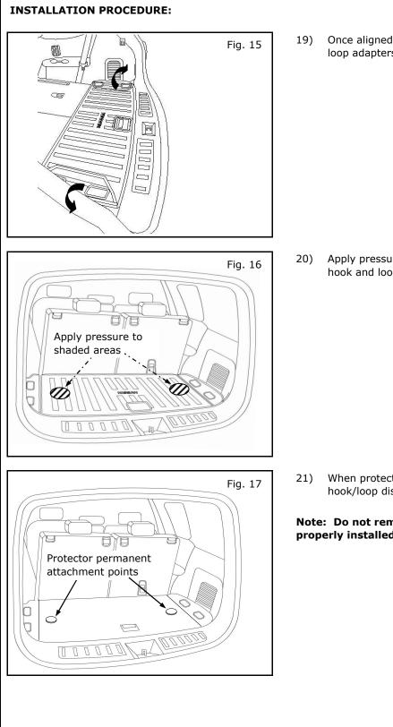
19) Once aligned, remove fingers from underside hook and loop adapters. Fold down side flaps.
