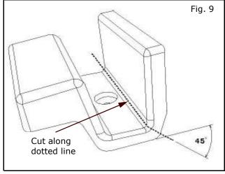
10. Cut plastic cover along dotted line at  $45^{\circ}$  as shown in Fig 9.
