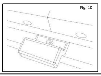
11. Re-install plastic cover onto center bracket.
