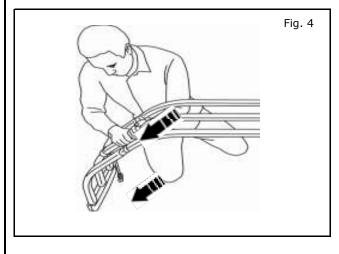
Note the unpainted section of the tubes. This will be used as a guide to assemble the tubes together. Figure 1 shows the intersection point of the center tube.
