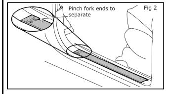
b) Lift kick plate from rear to front, disengaging from clips. Separate the Kick Plate from dash side panel by pinching the fork and sliding the kick plate rearward.
