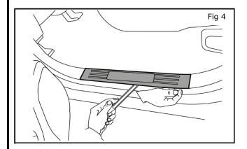
4) Removal of existing kick plate. Insert plastic trim removal tool under kick plate. Carefully Loosen and lift kick plate for removal, disengaging push pins.
