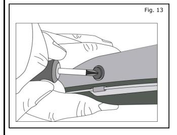
23) Squeeze hood protector to hood to eliminate any gap while fully tightening each screw.
