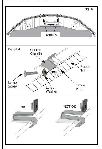
13) Slide center clips (B) onto hood under rubber trim and secure using the large screw through large washer, rubber trim and brackets into previously installed screw plug.
