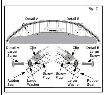
14) Secure left and right clips (C) onto hood under rubber trim and secure using large screw through large washer, rubber trim and brackets into previously installed screw plug.
