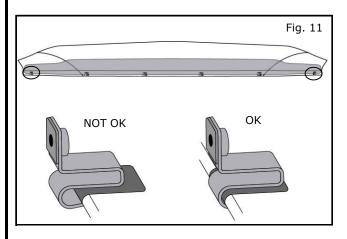
20) Install the wing clips "D" over the abrasive resistant tape strips at the previously marked locations.
