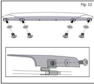
21) Insert small screws through fibre washer, loosely secure hood protector to outer clips "C" and wing clips "D".
