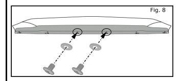
16) Insert small screws through fibre washer, loosely secure hood protector to center clips "B".
