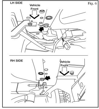
8) Install one locator bolt at each side(see figure 6).
