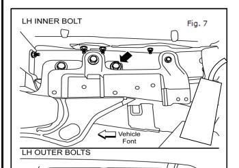
9) Install remaining three bolts at LH side(see figure 7).
