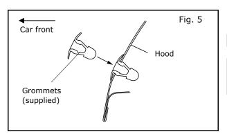
k) Install the grommets(supplied) in the drilled holes. See Fig. 5.
