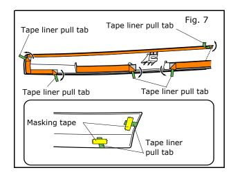
b) Fold tape liner pull tabs onto the hood molding accent painted surface and apply masking tape to ensure that the pull tabs are accessible. See Fig. 7.
