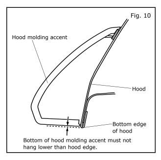
f) From the side of the vehicle, align the end of the hood molding accent to match the contour of the hood. See Fig. 10.
