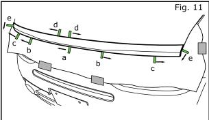
g) Starting at the center and moving outward, remove the double-sided tape liner a through c and apply at least 15lbs. of pressure to the hood molding accent to ensure that the hood molding accent is attached. See Fig. 11.
