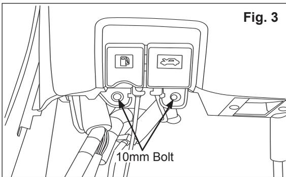
3) Remove driver side instrument lower panel.
