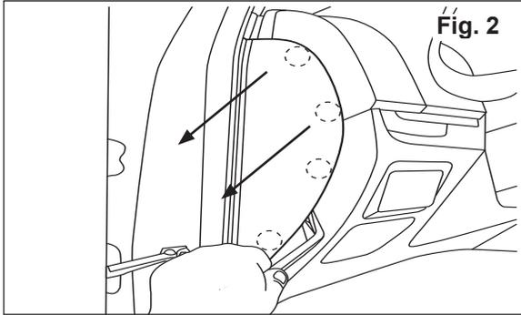
2) Remove driver side instrument side mask.
