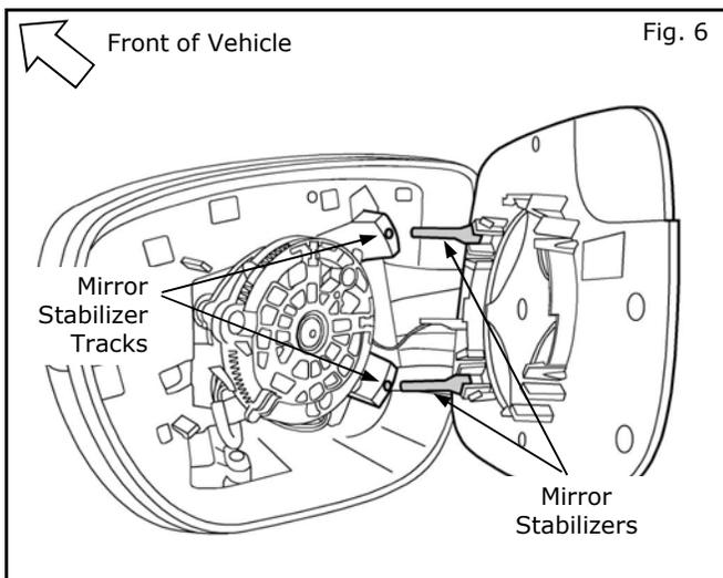
6) During installation, be sure that the two **mirror stabilizers** are lined up with the two stabilizing tracks in the mirror housing as the mirror assembly is placed into position over the glass actuator.
