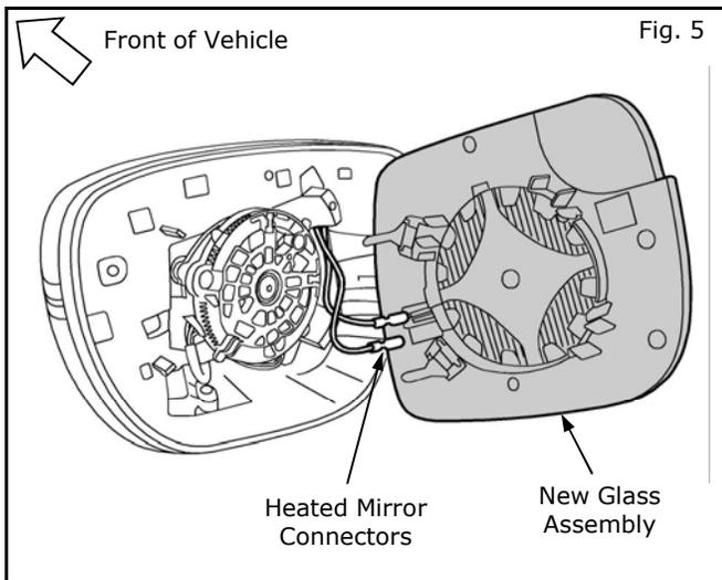
5) Begin installation of the new Blind Spot Mirror Glass Assembly by reconnecting the heater wires if necessary.
