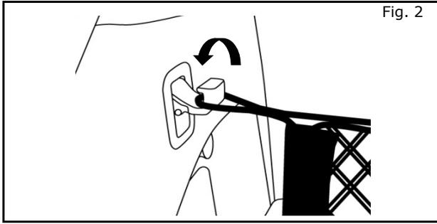
3) Attach net loops to upper hooks (driver side shown).
