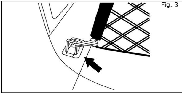
4) Attach net hooks to lower clips (driver side shown).
