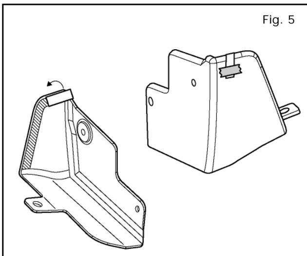
7) Fold tape liner pull tabs onto front splash guard surface and apply masking tape to ensure that pull tabs are accessible.
