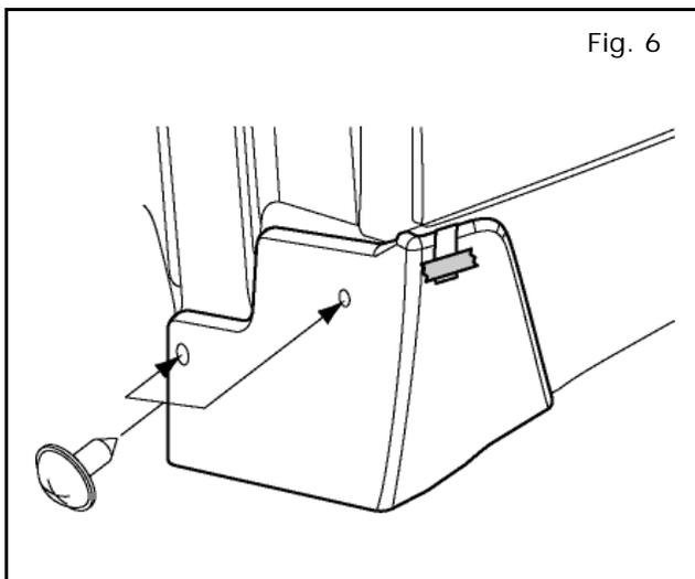
8) Align front splash guard to vehicle and loosely install phillips screws (E) making sure pull tab is exposed.
