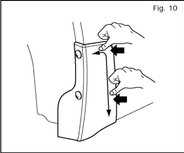
11) Apply at least 15lbs of pressure to rear splash guard to ensure that tape is attached.
