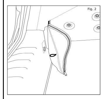
2) Attach pouch to drivers side anchors, un-zip pouch and un-roll net to attach to passengers side of vehicle.
