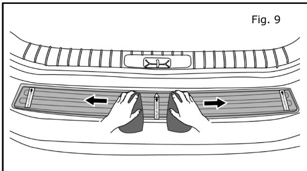
13) Using clean, lint-free cloth, start at center and apply 15 lbs/in of pressure along tape path.
