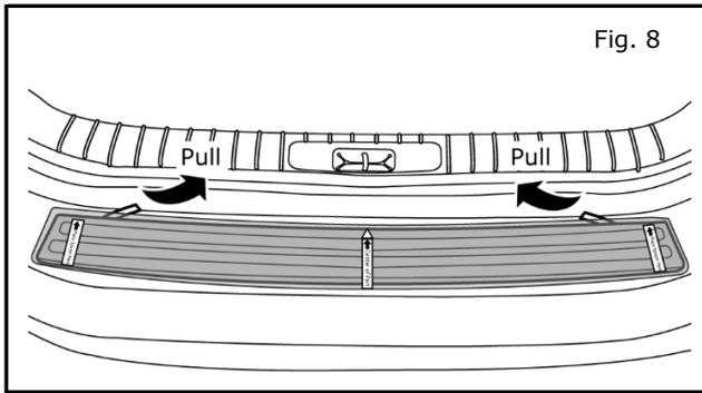
12) Remove front tape liners by pulling at a low angle.
