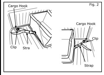
3) Secure Cargo Organizer to Cargo Hooks located on floor of vehicle using (2) straps with clips (Passenger rear attachment shown).
