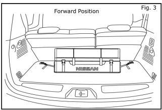
3) Cargo Organizer can be secured to either the forward Cargo Hooks (see Fig. 3) or the Rear Cargo Hooks (see Fig. 4).
