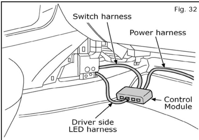
32. Route the harnesses under the center stack. Plug all harnesses into the control module.
