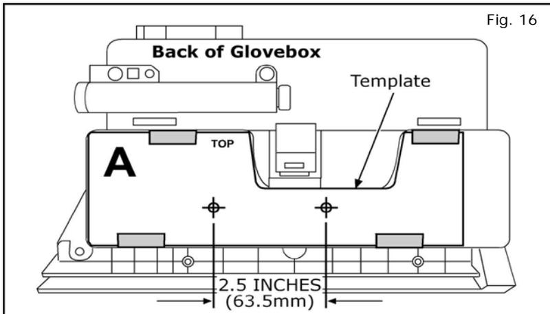
16. Trim out template "A" and tape in place on back of glovebox as shown. The template should be positioned along the bottom and left edge with the letter "A" in the upper left hand corner.
