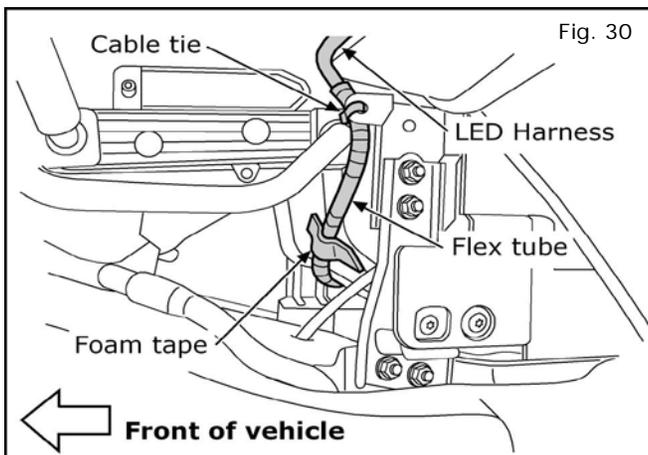
30. Route driver side harness through the center stack and out towards the passenger footwell. Secure with a cable tie and foam tape as shown.
