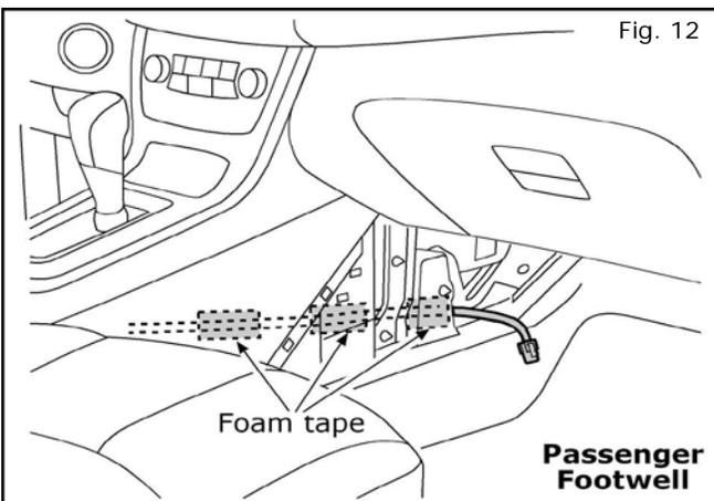
12. Route encoder wiring harness up through the center stack and out to the passenger side footwell. Secure harness inside center stack with foam tape.
