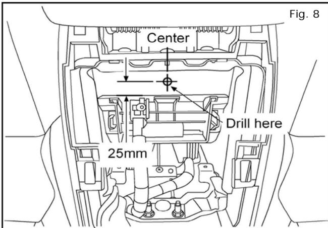
8. Measure and mark across the top of the storage compartment to establish center. Measure and mark 25mm (1") up from the bottom edge as shown.
