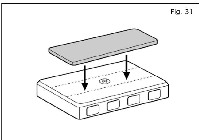
**Note: Attach one (1) 58mm x 82mm foam tape to the underside of the accessory control module, covering the screw in the center.**
