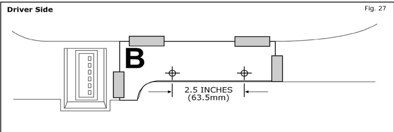
27. Trim out template "B" and tape into place on bottom of the steering finisher as shown. The template should be positioned along the bottom edge with the letter "B" on the left hand side.
