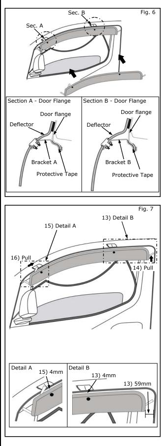
12) Attach deflector to door by sliding brackets onto door flange.
