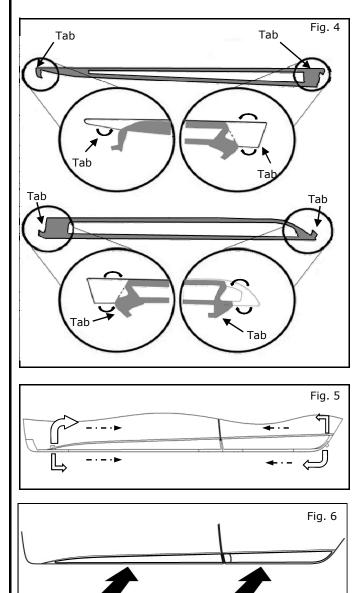
6) Using pull tabs, remove red tape liner from small tape on each end and approximately 30mm from each end of the long tape. (Fig. 4)
