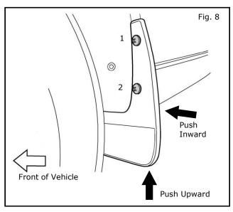
9) Push splash guard upward and inward towards vehicle and tighten screws in sequence shown.
