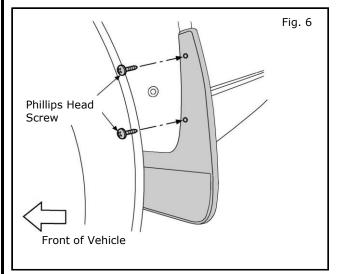
6) Align splash guard to vehicle and loosely install two phillips head screws.
