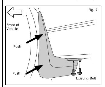
8) Push splash guard upward and inward towards vehicle and reinstall existing bolts.
