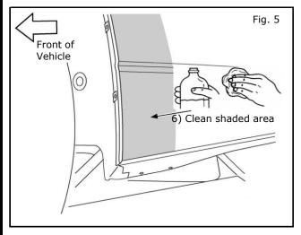
5) Clean installation surface (shaded area) with mild soap/water mixture.
