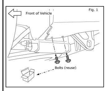
1) Remove 2 bolts from bottom of rear bumper (Keep to reuse).
