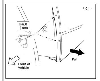
3) While pulling rear bumper outward, drill 6mm (1/4") holes at center of dimple mark locations on bumper.
