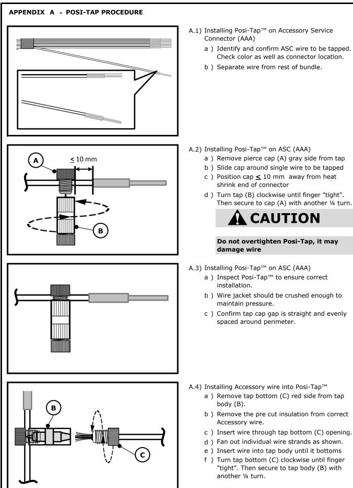
b) Wire jacket should be crushed enough to maintain pressure.
