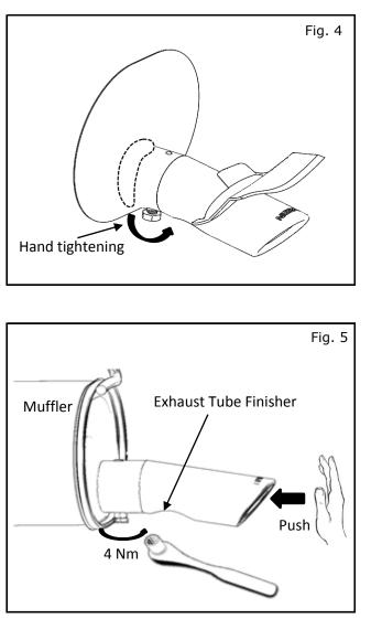
4) Adjust the exhaust tube finisher to contact the vehicle muffler wall. Lightly tighten bolt by hand, enough to maintain the part in place. See figure 4.
