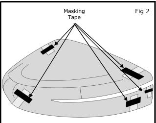
3) Fold pulling tabs and tape to outer surface of Mirror Cover (Fig.2).
