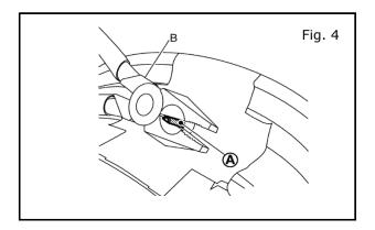
11) Cut roll pin (A) of valve, using pliers (B). See Fig. 4.
