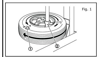
7) Turn tire so that valve hole is at bottom and bounce so that tire pressure sensor (1) is near valve hole. Carefully lift tire onto turn-table and position valve hole (and tire pressure sensor) 270° from mounting/dismounting head (2). See Fig. 1.
