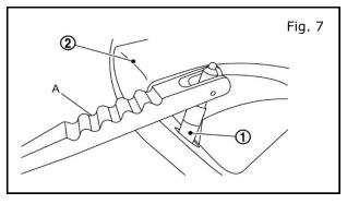
b) Intall valve (1) to road wheel (2), using valve inserter (A). See Fig. 7.
