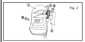
8) a) Remove stopper (2) in directions (A) using pliers. See Fig. 2.
