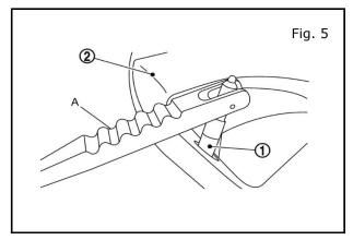
12) Remove valve (1) from road wheel (2), using valve inserter (A). See Fig. 5.
