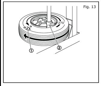
17) Set tire onto turntable so that tire changer arm (2) is at a position approximately 270 degrees from the tire pressure sensor. See Fig. 13.
