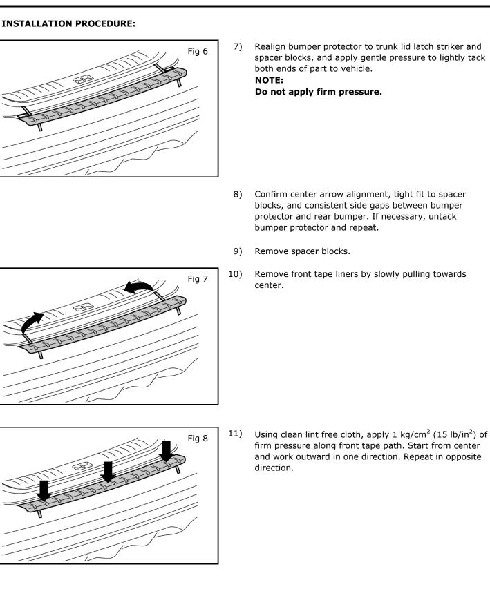
Realign bumper protector to trunk lid latch striker and spacer blocks, and apply gentle pressure to lightly tack both ends of part to vehicle.
