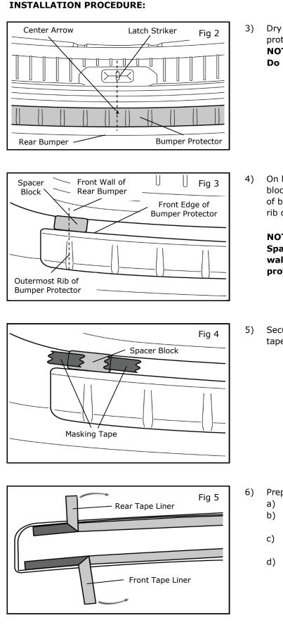
Dry fit bumper protector on vehicle. Align bumper protector center arrow with trunk lid latch striker. NOTE:
