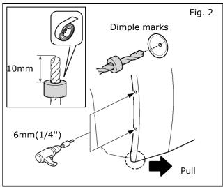
2) Pull out on bottom corner of rear bumper, and drill 6mm(1/4") holes at dimple locations.
