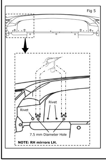
7) Enlarge 8 pilot holes shown with 8 mm (5/16 inch) drill bit.
