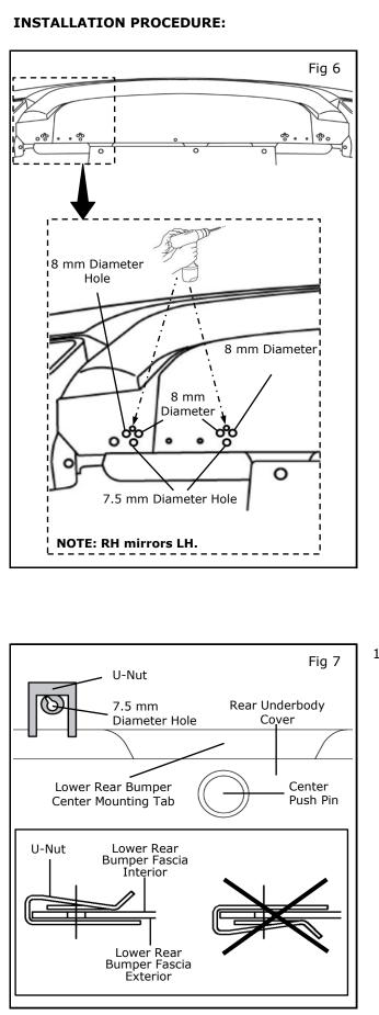
8) Enlarge 4 pilot holes shown with 19 mm (3/4 inch) spade bit.
