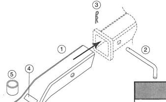
Insert Draw Bar(#1) into receiver opening. Line up holes on receiver with holes on Draw Bar and push Pull Pin(#2) through opening. Insert Clip(#3) through hole in Pull Pin. Be sure clip is fastened securely.
