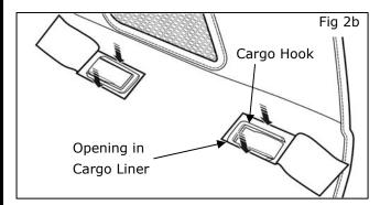
Align openings in liner with cargo hooks located in the floor in back of vehicle.
