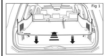
1) Open the rear door and fold down the third row seats. Locate the front edge of cargo liner and place the front edge on top of the 3rd row seats.
