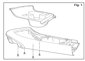
1) Remove (4) Phillips screws attaching Cupholder.
