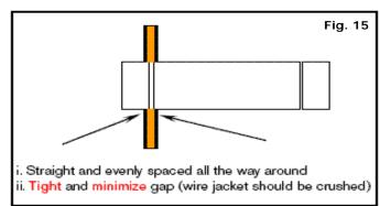
15) Inspect the tap to ensure correct installation.
