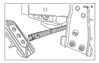
9) Route Passenger side light assembly behind IP brace as shown.
