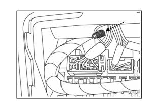
w) Spread wires with fingers exposing the Violet / Yellowstriped wire and attach grey cap of Posi-tap. (Use shop light to illuminate the area)
