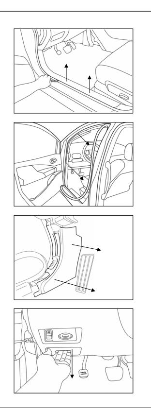
b) Using panel removal tool, disengage clips on driver-side scuff plate and remove.
