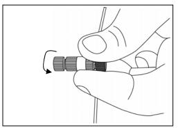
x) Attach body of Posi-tap to grey cap by twisting until securely tightened.
