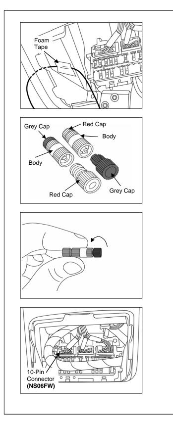
s) Secure EC harness power wire with 1 piece of foam to center dash frame.
