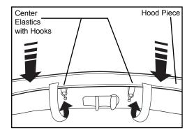
Open hood and attach center elastics with hooks to holes located on either side of center hood latch opening. Be sure that hooks go into hole in second layer of sheet metal. Slip hood piece onto each corner of the hood and pull taut.
