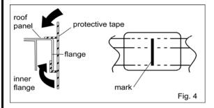
Attach a piece of protective tape to the roof at each of the marked locations using the marks as centerlines. Wrap the protective tape around the bottom of the sheet metal flange, making sure it does not contact the inner sheet metal flange
