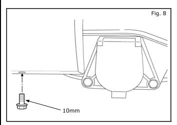
8) Re-secure the bumper trim with the 10mm mounting bolt from Step 2.
