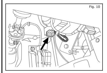
10. The connector for the controller unit jumper is located under the steering column, next to the diagnostic connector. Carefully cut away the tape at the harness to access the connector.
