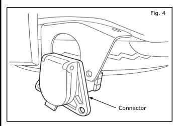
4. Slide the connector approx. 3/4 of the way onto the mounting bracket. This will allow space for mounting the second bracket bolt.
