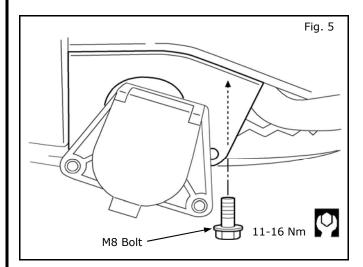
Rotate the mounting bracket into final position and align the mounting hole. Install the second M8 bolt and torque both bolts to 11-16 Nm.
