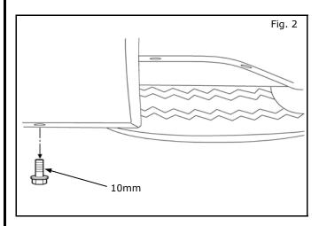
2. Locate the hex head bolt on bottom of the bumper trim to the left of the mounting area. Remove the bolt using 10mm socket wrench (save the bolt for later reinstallation).
