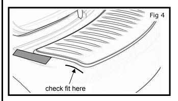
5) Check the fore/aft alignment of the bumper protector to the curvature of the bumper for consistent gap. See Fig. 4.
