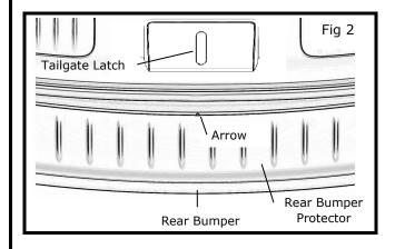
3) Dry fit the bumper protector on the vehicle .a) Align the bumper protector centering
