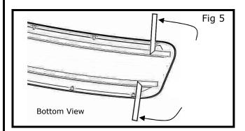
6) Remove part and peel back approximately 30mm on all tape liners. See Fig. 5.
