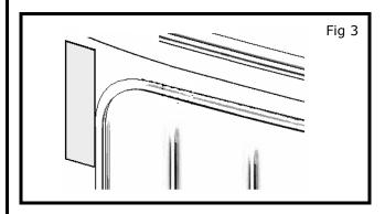
4) Apply locating tape to bumper at right & left edges of the part. See Fig. 3.
