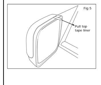
4) Align the top and outboard edges of the mirror cover to the mirror housing ensuring uniform spacing to the edge of the mirror housing.
