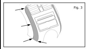
5) Carefully and lightly place part in position by aligning cluster finisher - LH edge with dash edge surrounding cluster of the vehicle.
