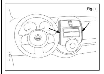
1) Use an alcohol wipe to clean the indicated areas on the vehicle where the cluster finishers (LH and RH) are to adhere.
