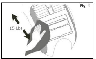
6) Once cluster finisher - LH is adjusted to the correct position, use clean towel and apply minimum 15lbs of pressure over entire surface, for at least 30 seconds.
