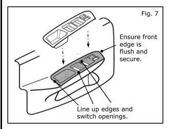
13) Carefully and lightly place part in position by dropping it straight down without bending or twisting. Once in place, make sure all switches operate correctly with no obstructions.
