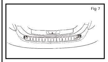
Place part back on vehicle and align it to all masking tape edges.
