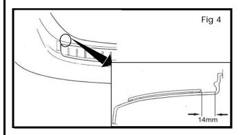
5) Measure the distance from the corner radius of the rear bumper fascia to the edge of the bumper protector (14mm).
