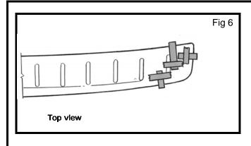
7) Remove part from vehicle. Fold the clear tabs over the edge of the part and secure to the top surface with masking tape.
